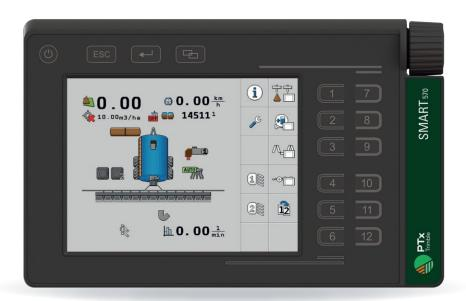
The SMART570 offers a capacitive 5.7 inch (14.5 cm) touch screen for on screen control, 12 programmable softkey membrane buttons for operation while on the move, and a rotary encoder for rapid changes of numerical data. The SMART570 is also capable of displaying machine and implement data when multiple ECUs are attached.
